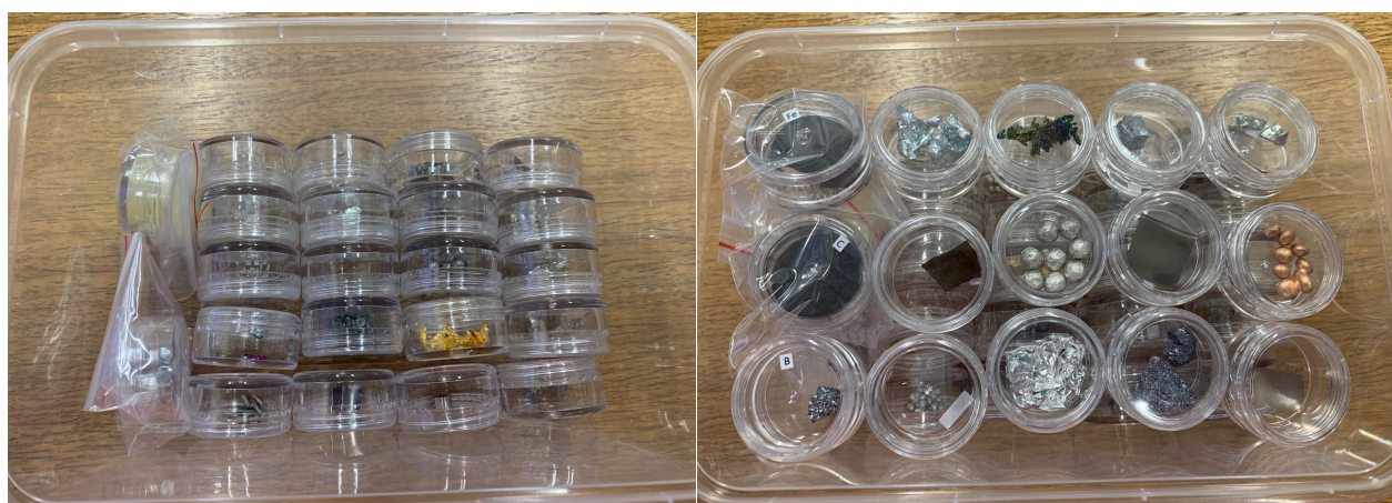
Best way to pack the samples – 22 samples on the bottom layer (left), followed by 15 samples on the top layer (right).
